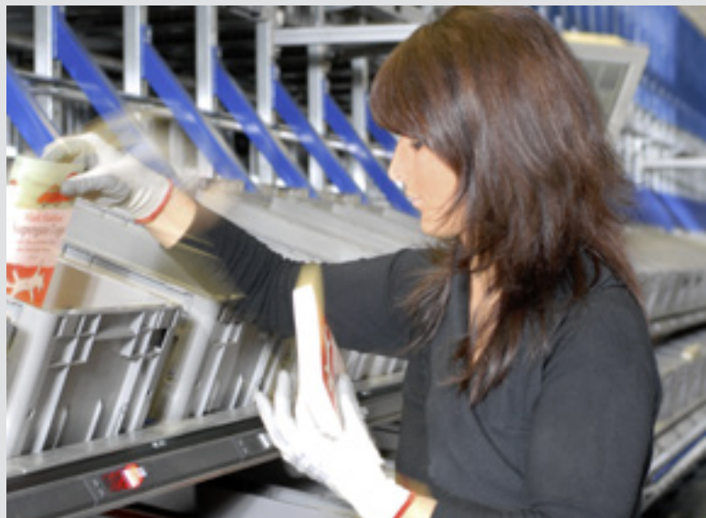
▲ The containers' smooth interiors enable quick, manual picking
