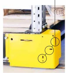
**Component protection** Effective component protection: Light barriers and proximity sensors protected under rugged cover.
