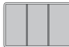
3-way crosswise partitioning* Compartment size: 182 x 366 mm
