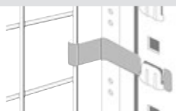
Mesh back panel fastening
